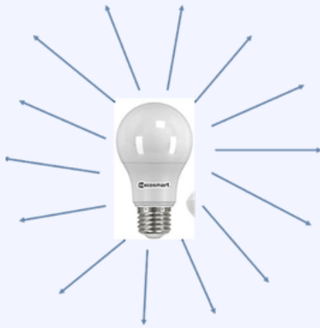
Figure 3 : A conventional light source emits uniformly in all directions, covering the full 4\pi solid angle. This figure presents a 2D view of a typical LED bulb, illustrating light rays radiating outward in every direction.
